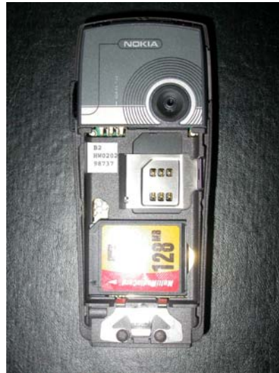
Figure 11: MMC Card Placement
